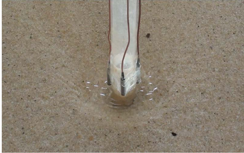
Figure 7. Picture of the scour hole at the end of the experiment ( t=360 s)
