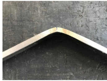
Figure 10. Macrograph showing the failure location in root bend specimens extracted from the higher heat input joint. Note that failure takes place in the coarse grained HAZ (CGHAZ) region.
