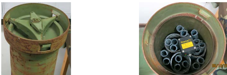
Figure 9. Propelling charge for ammunition 155mm, Metal container
