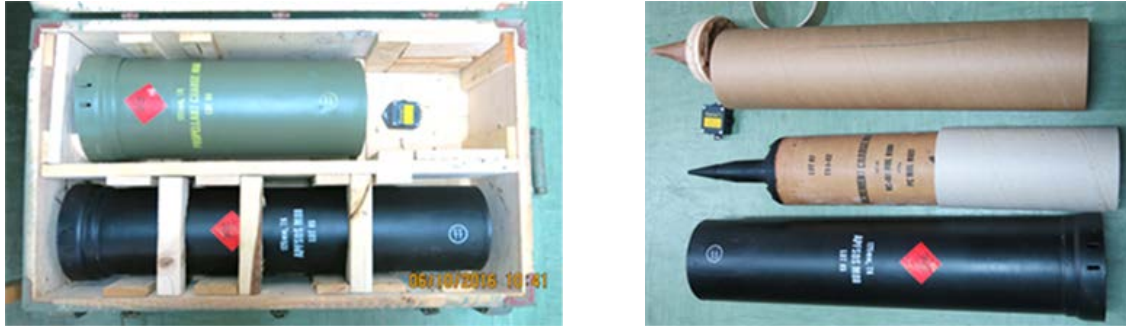
Figure 7. Tank ammunition 125 mm, APFSDS-T, M88, packaging
