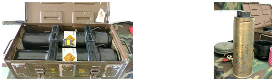
Figure 3. Cartridge propelling 105 mm, L35, packaging
